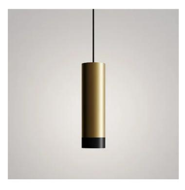
Suspension lamp in anodized aluminum (available in two finishes: gold and silver) with a PMMA lens. The LED light source is available in two color temperatures: 2700 or 3000 K. The lamp is also designed for modular use; the end of the lamp features an anti-glare black anodized nut, which can be replaced with borosilicate glass elements, giving rise to the Sfera & Sfer'Otto collection. Suitable for indoor use only.
